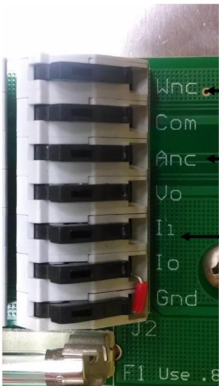
From DCSAP "Wnc" to WATCHMAN TB2 "S2" Green Wire (Wnc=Warning normally closed contact)
